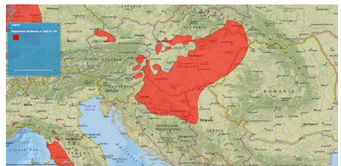
Figure 4: Temperature distribution map at depth of 2000m in the Pannonian Plain (temp. > 90°C)
